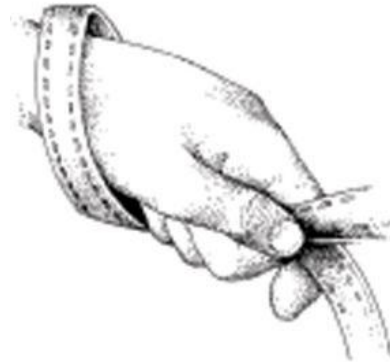
Incorrect method of holding the lead line
